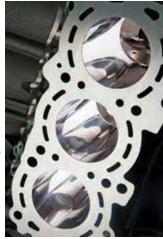
Graphical representation of the cylinder finish, such as that displayed on an Abbott-Firestone Curve, provide a qualitative analysis of the characteristics of the surface finish. The Rk family of parameters directly analyzes the surface characteristics over a given sampling length.
